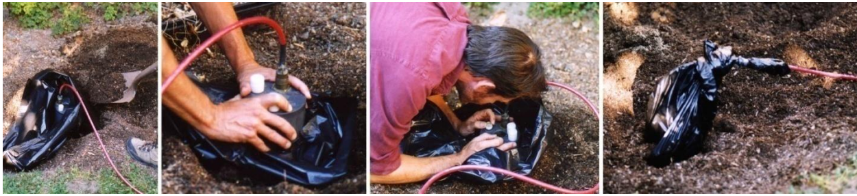
Figure 7. MT magnetometer installation – bury in bag, align, level, and bag connector.
